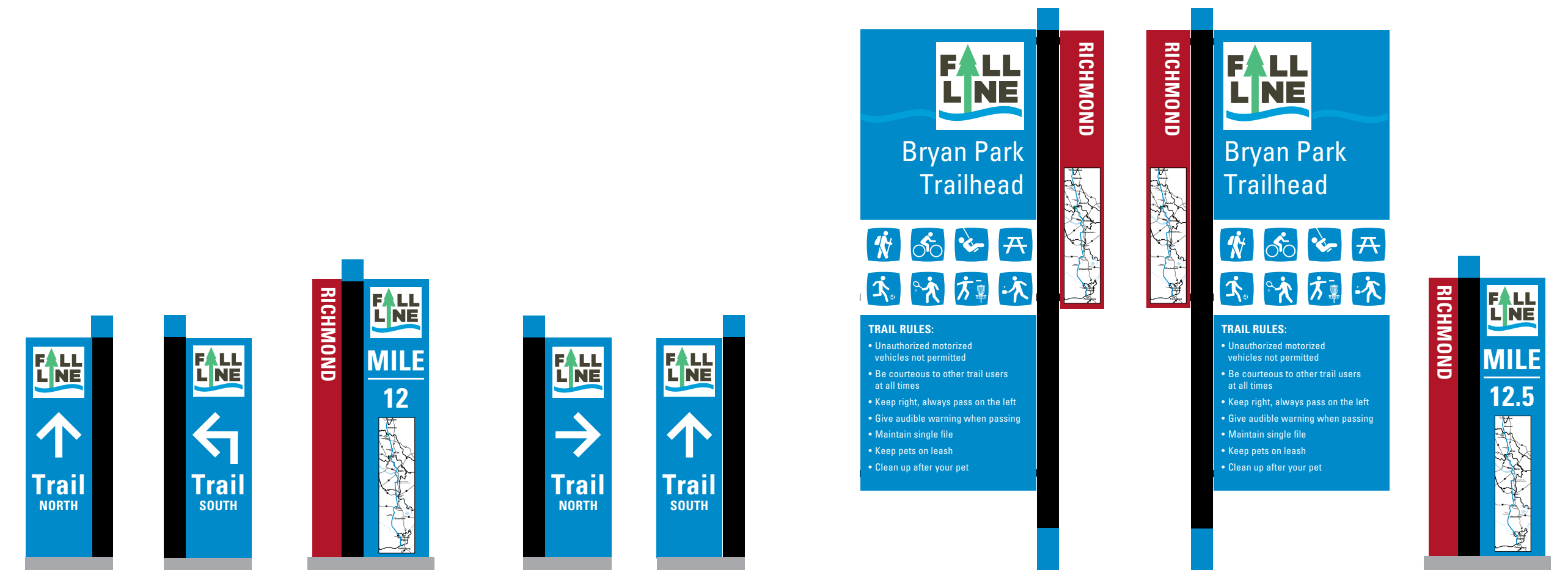
Sign Type W.42A Directional Sign W.42B Sign Type M.12 Mile Marker Sign Type W.43A Directional Sign W.43B Sign Type T2.41A Pedestrian TrailRad/Regulatory Sign Sign Type T2.41B Pedestrian TrailRad/Regulatory Sign Sign Type M.12.5 Mile Marker
